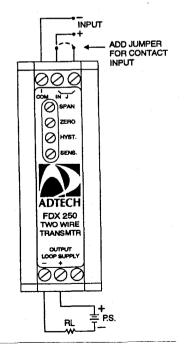
NOTE: For contact input connect a jumper as shown dotted
